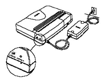
When the battery is fully charged, the CHARGE light turns off.
